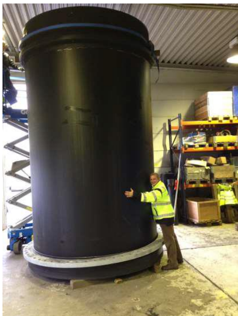
Photo 1 - The 2.5m diameter pipe section
