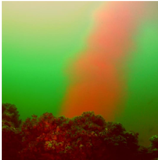
Photo 7 - Dye coloured Brine Jet using Rhodamine WT injection
