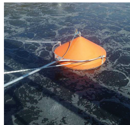
The Alphameter helps engineers understand how the alpha value in an AS system constantly changes
