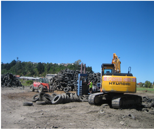
Photo 7: Baling selected tyres on site
