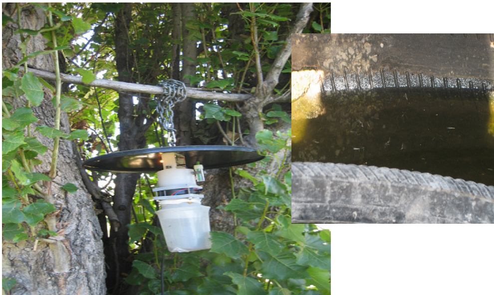
Photo 12: Light trap for mosquito surveillance (inset: mosquito larvae in tyre on site)
