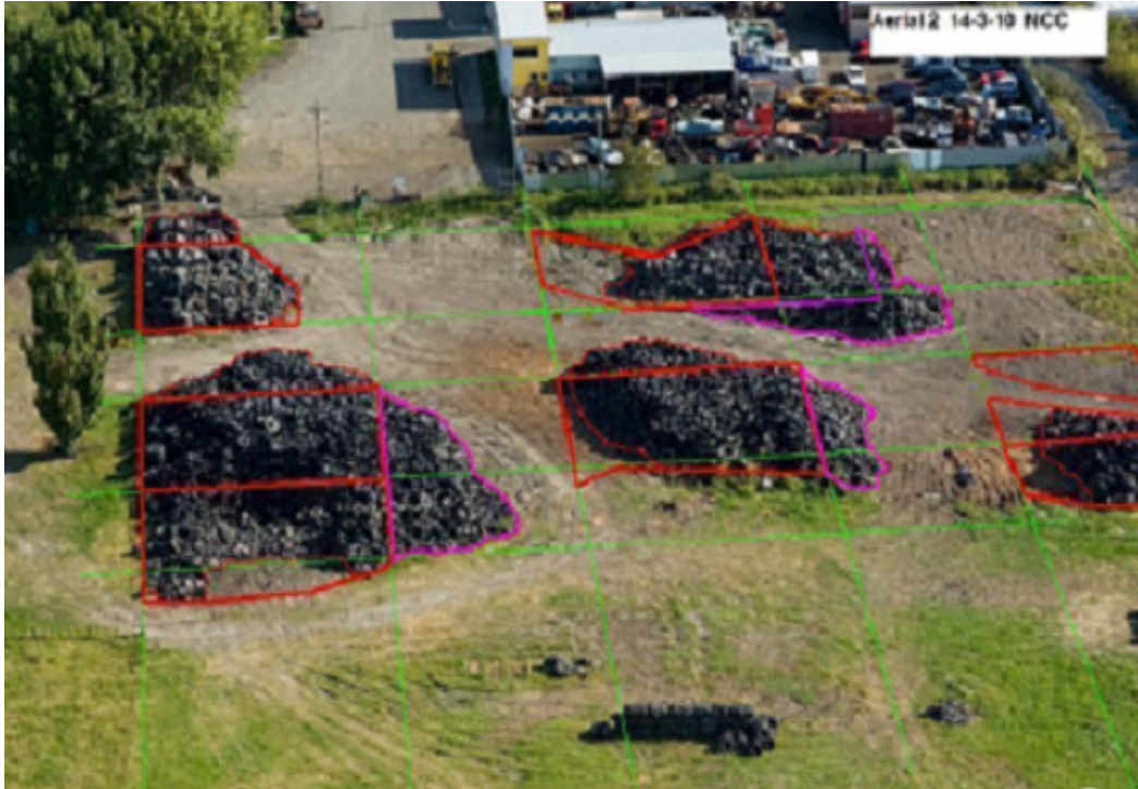
Photo 4: In-situ pile disaggregation creating the fire break grid and smaller piles
