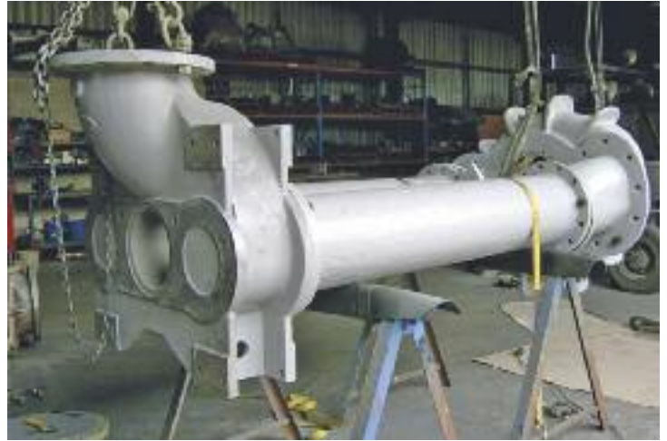
External surface protected against high temperature with Belzona
