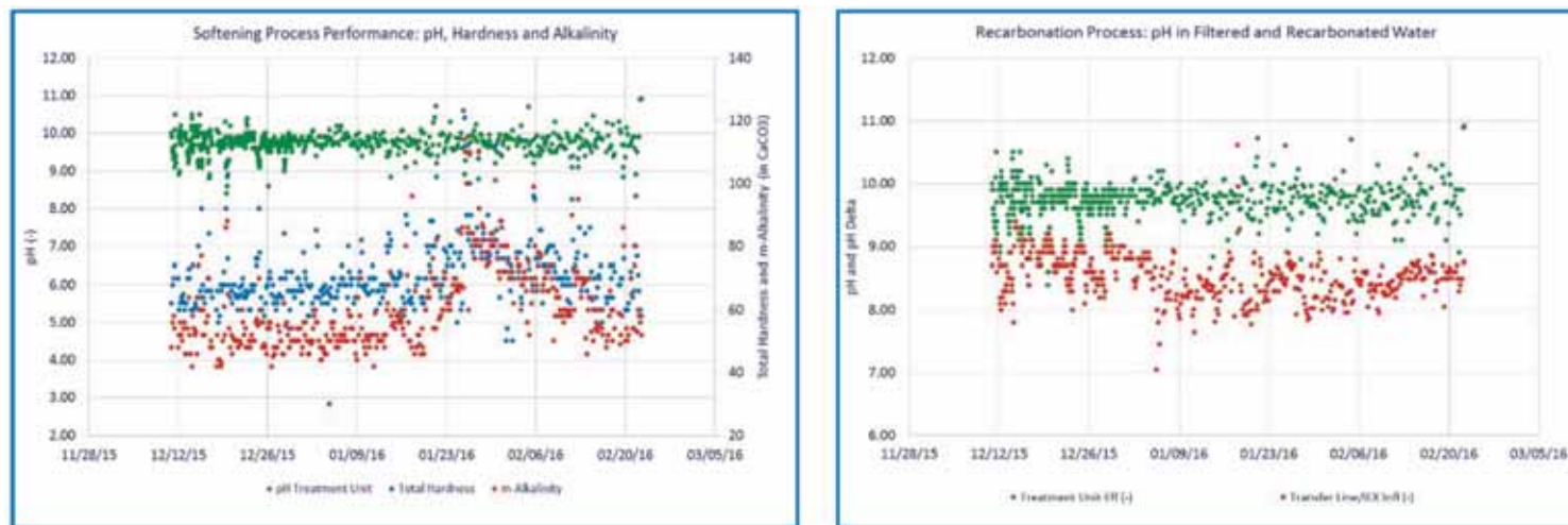
Figure 5. Softener Effluent pH, Hardness and Alkalinity (left), pH Before / After Recarbonation (right)
